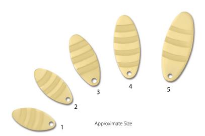
This blade is shaped the same as the Swing blade on page 72, with the exception of the finely detailed ripple effect stamped into the blade. Ripple blades have excellent reflective qualities and spin very freely. Stamped from solid brass, all polished and plated finishes are free from sharp or rough edges.
