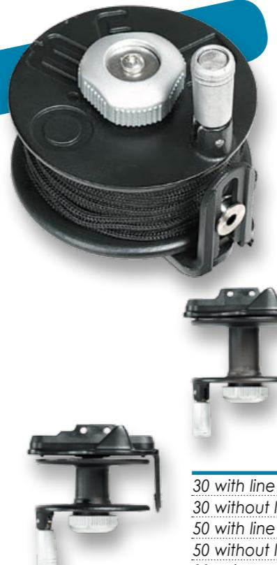
"Half enclosed" reel available in two versions: 30 or 50mt 1.5mm line capacity. Extendable handle to reduce the size of the reel and steel sliding line guide. The spool has two bushes which eliminate the friction on the spool shaft. Complete with a drag system which keeps the line in tension even with the friction completely open.
